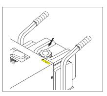
**STEP 1:** Check fuel tank and pump oil levels on both machines and connect garden hose to pressure washer. **CAUTION:** Only use fresh water to this machine.
